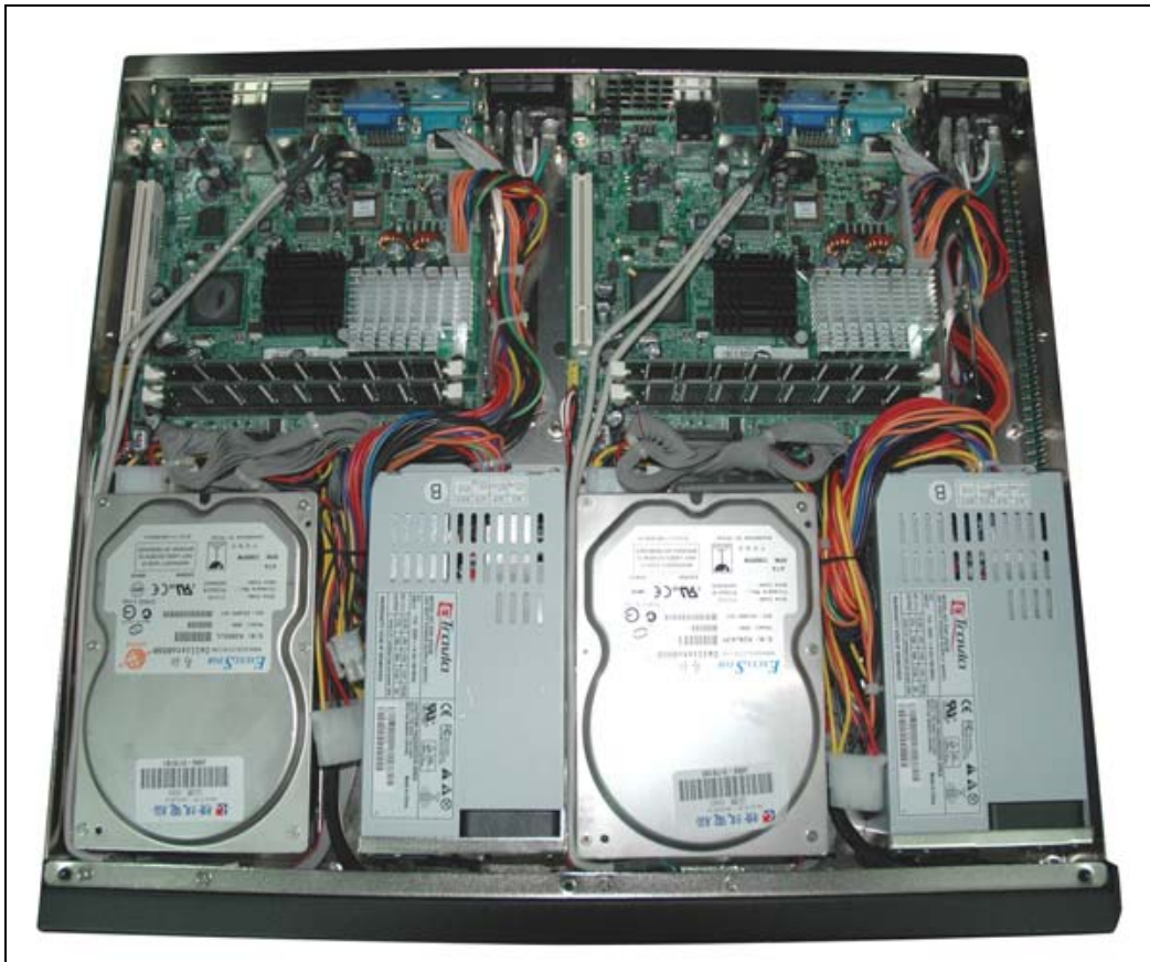
Figure 7: 1U Server with Dual VIA VT310-DP Mini-ITX Mainboards and Dual Hard Drives
