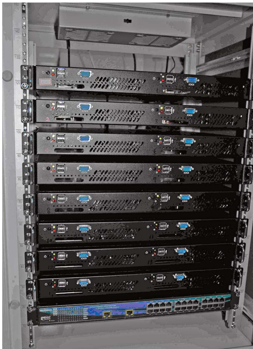
Figure 9: 16-Node Cluster in 8 x 1U units Based on the VIA VT310-DP Mainboard
